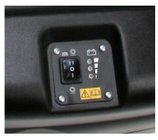
A single switch and battery level indicator allows for minimal operator training.
